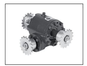
The GWK-serie, with self-braking worm wheel transmission (reduction i=35), is used, among other applications, in continuous ridge ventilation systems or panels in stables.
