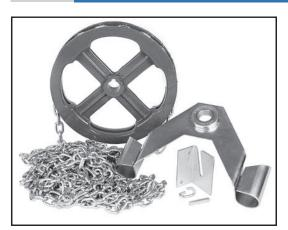
The chain pocket wheel is used to drive the GWK240 and GWK400 worm gearboxes by hand. The chain pocket wheel set consists of a pocket wheel, an 8 meter chain with connecting link and chain guidance. The pocket wheel is mounted on the ingoing axle of the worm gearbox. On site the chain can be adjusted to length.
