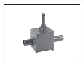
The HKK120 distribution gearbox (1:1) is used in the THG30 drive system. The ingoing shaft of the HKK120 is hollow so it can be mounted over the 1" tube driven by a GW motor gearbox. The tube has to be fixed with 2 M8 bolts. The drive tube is branched off at a 90° angle in the gearcase, for example to drive a GWK worm gearbox.
