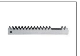
The gear rack for the THG30 rack box is manufactured from sendzimir galvanised steel plate. The rack is 30 mm in height, and has a wall thickness of 2 mm. The rack is fitted with a run-out safeguard to prevent the gear rack from running out of the gearcase. The rack is also fitted with a blow-out safeguard to prevent the gear rack from blowing out when it is in the run-out safeguard position.
