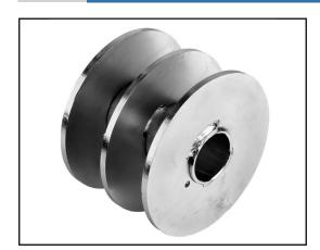
The double winch drum is suitable for mounting over a 5/4" drive tube. The galvanised winch drum is fixed with two spring dowel pins and can be used for hoisting drinker- or feeder lines. Multiple which drums can be placed on one 5/4" tube which is driven by a GW gearbox.
