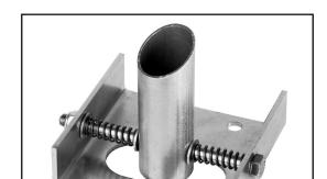
The galvanised mounting bracket for the GXP10 guidance, is used to fix the Ø32 mm guiding tube of the GXP10 to the floor. The spring construction allows the tube to move laterally and with that it allows the roll tubes to expand.
