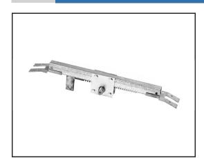
The THG10S is a rack box specially developed for swinging ventilation systems in Venlo greenhouses. The rack box is driven by a GW motor gearbox and drives the swing tube by means of a gear rack.
