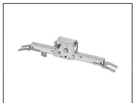
The THG24S is a rack box specially developed for swinging ventilation systems in Venlo greenhouses. The rack box is driven by a GW motor gearbox and drives the swing tube by means of a gear rack.
