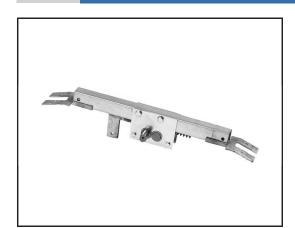
The THG10SC is a rack-and-pinion drive specially developed for swinging ventilation systems in Venlo greenhouses. The gear rack of the THG10SC operates in the opposite direction to that of the THG10S. This makes it possible to use one GW motor gearbox to drive the ventilation windows on either side of the ridge.
